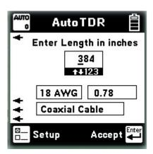
The Auto TDR function imports the coaxial configuration selected in the TDR function using the Setup key.
